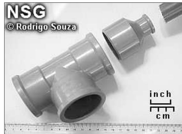
Materials: (1) a 2" or 3" T-joint; (2) a 2" or 3" × 1" coupling; (3) about 3' of 1" pipe for the handle; (4) PVC glue/cement.
